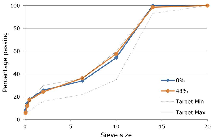
**Figure 1 Grading envelope and achieved grading for 14 mm SMA with addition of RA at 0% and 48% by mass**
