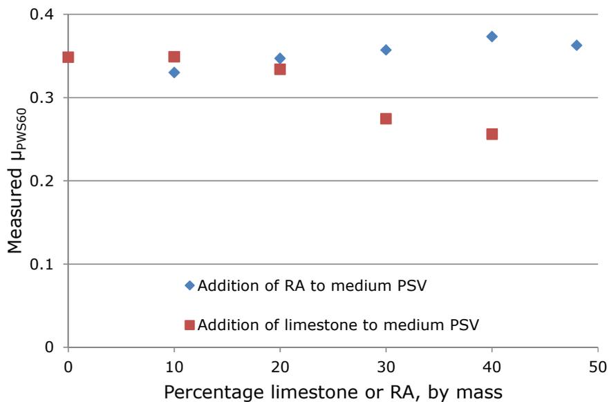
**Figure 2 The effect on friction of adding RA or limestone to an SMA**
